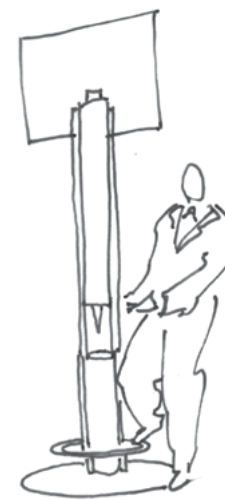
Entry-scaled Hand Hygiene Station with Signage
